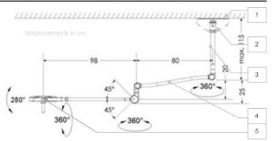
If fixture is to be installed above a drop ceiling, Additional items 6 or 7 must be ordered separately. Please refer to Triango Pre-Install Guide for installation suggestions.
