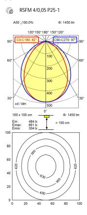
light sourceLEDwork equipmentwithoutconnected load20-28V, DCpower consumptionenv. 14 Wluminous fluxapprox. 1.450 lmluminous efficiencyapprox. 104 lm/W
