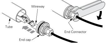
2. Rotate end cap so lamp is oriented correctly. The end cap must be against the tube so there is no gap between the tube and end cap.
