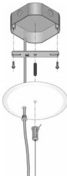
Typical Installation w/ Canopy Kit Option
