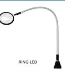
Voltage: Lamping: Operation: Magnification: Lens Cover: Protection Rating: Arm System: 120V or 240V, 50/60Hz 6 x 1W LED Includes touch switch 5.3 diopters Clear acrylic IP20 15.7in (400mm) gooseneck arm
