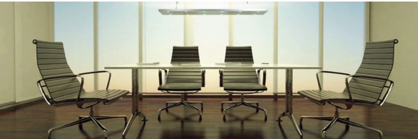
A warm relaxed scene, thanks to the high proportion of indirect illumination from T5 fluorescent lamps.
