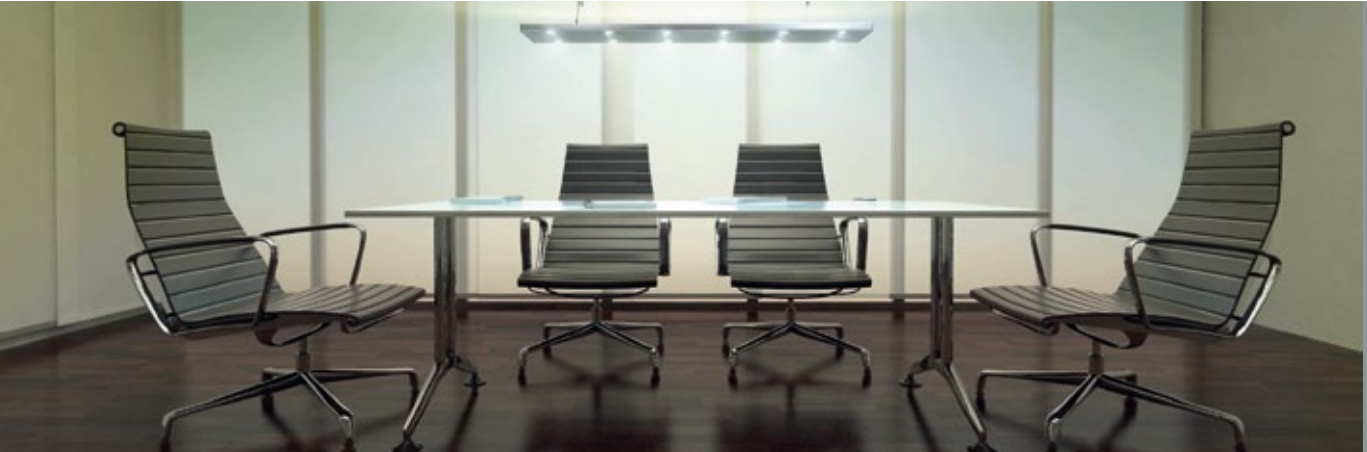
A balanced, comfortable lighting scene with an even distribution of direct light from LEDs and indirect light from T5 fluorescent lamps.
