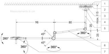
If fixture is to be installed above a drop ceiling, Additional items 3 and 4 must be ordered separately. Please refer to Triango Pre-Install Guide for installation suggestions.
