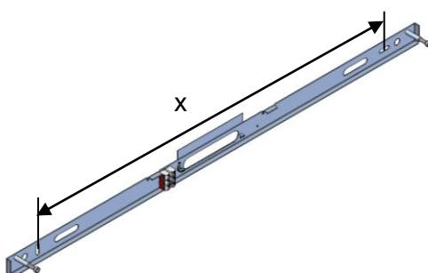
Fix the wall rail with the enclosed dowels at a applicable wall.
