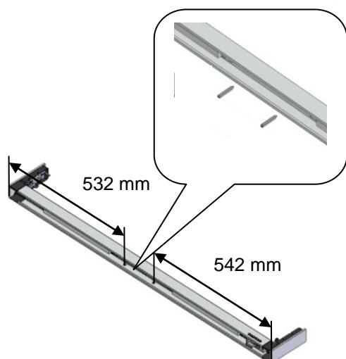
Screw the distance bolts into the middle float according the drawing.
