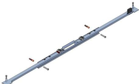
Fix the rail with collision micro switch with the enclosed dowels at a applicable wall. Distance of the bore hole is 510 mm.
