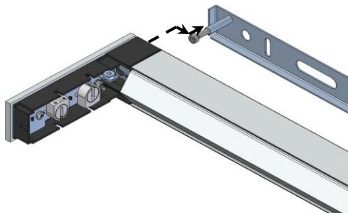
Loose both flat head screw of the face plate and remove the face plate. Remove the fluorescent lamps und fit the lamp according picture.
