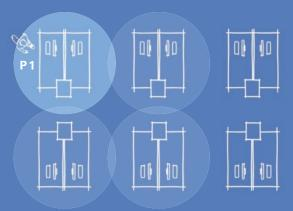
**Group 1.** The luminaire detects Person 1 and switches itself on. The work station of Person 1 is illuminated with its work level. The neighboring luminaires also switch on with basic brightness in support.
