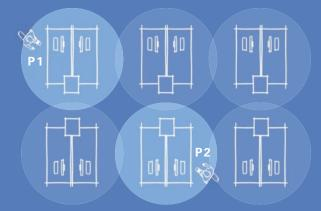
**Group 2.** The luminaire detects Person 2 and switches itself on. The work station of Person 2 is illuminated with its work level. The neighboring luminaires also switch on with basic brightness in support.
