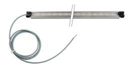
LED fitted with work equipment without connected load 24 V, DC power consumption approx. 2.8 W luminous flux approx. 252 lm luminous efficiency approx. 90 lm/W
